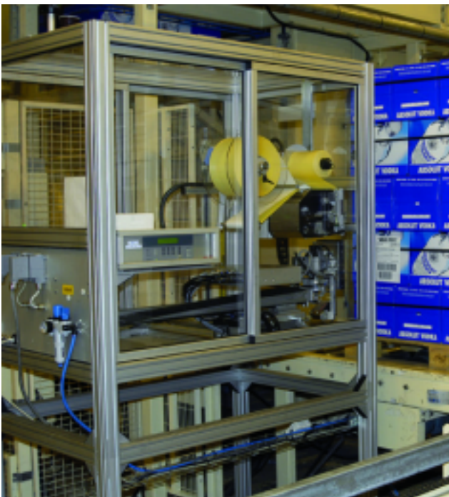
M200P pallet applicator with bar code validator
