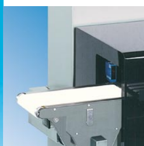
Variability Transport direction and line height can be set
