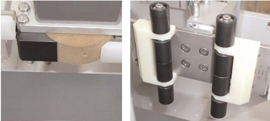
Roller-type separator and roller prism of model HERMA 152 C Prisma, easily adjustable
