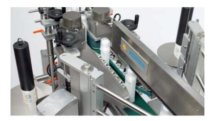
Products being separated, aligned, and stabilized.
