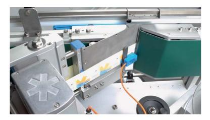
Another advantage: the label recognition unit does not need to be adjusted for different label formats.
