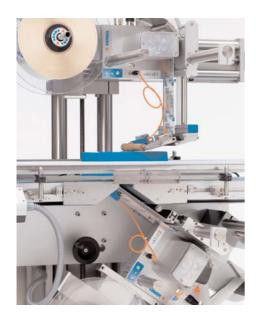
Top and bottom labeller: completing the job in a single pass.
